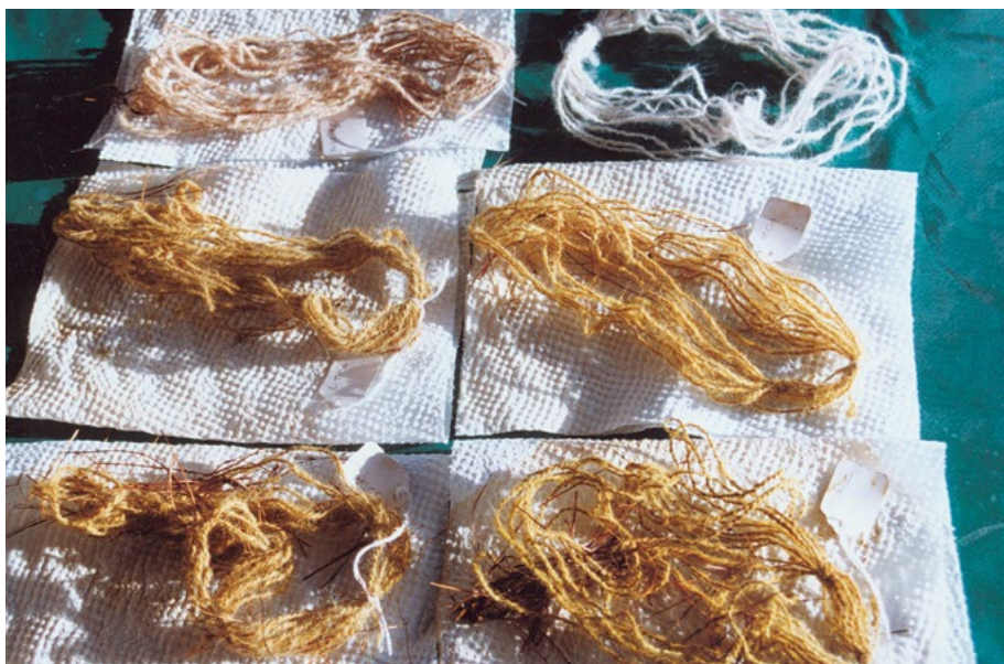
The dyed, dried, unrinsed skeins. Left to right and top to bottom: well water, undyed control skein, lithia water, iron water, soda water, and arsenic water.
