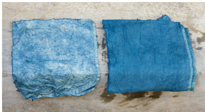
A single length of cloth torn in two. Scoured on the right, not scoured on the left.
