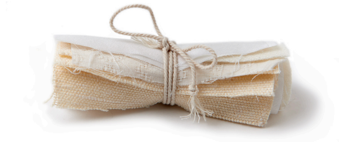
A single length of cloth torn in two. Scoured on the right, not scoured on the left.
